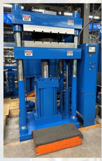
As part of our planned Phase I expansion, Diacom Corporation is pleased to announce the purchase and installation of a new 300-ton press with 36" platens. The new press will help DiaCom further serve our customers in oil and gas, nuclear, and water control industries by manufacturing larger size diaphragms.
