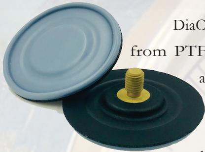
DiaCom has capabilities to design and manufacture composite diaphragms made from PTFE/Elastomeric materials capable of standing up to even the most chemically aggressive of environments. DiaCom's process bonds PTFE, ranging in thickness from .002" up to .040", to rubbers of varying characteristics. DiaCom's unique process and construction produces a diaphragm that is compatible with these harsh environments without limiting the life and responsiveness of the diaphragm.
