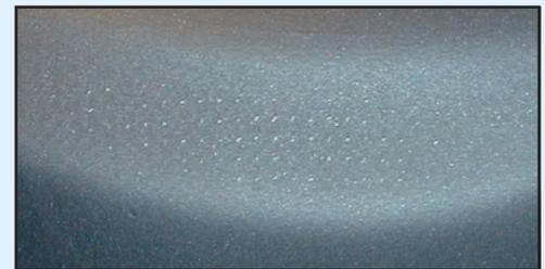
Inverted Head Radius of a Top-Hat Diaphragm.
